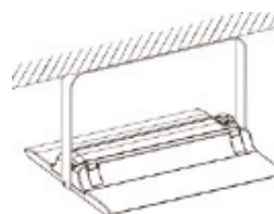
Suspended fixing by U-shaped bracket
